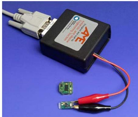
**Figure 22 - Interface box connected to a geolocator.**
