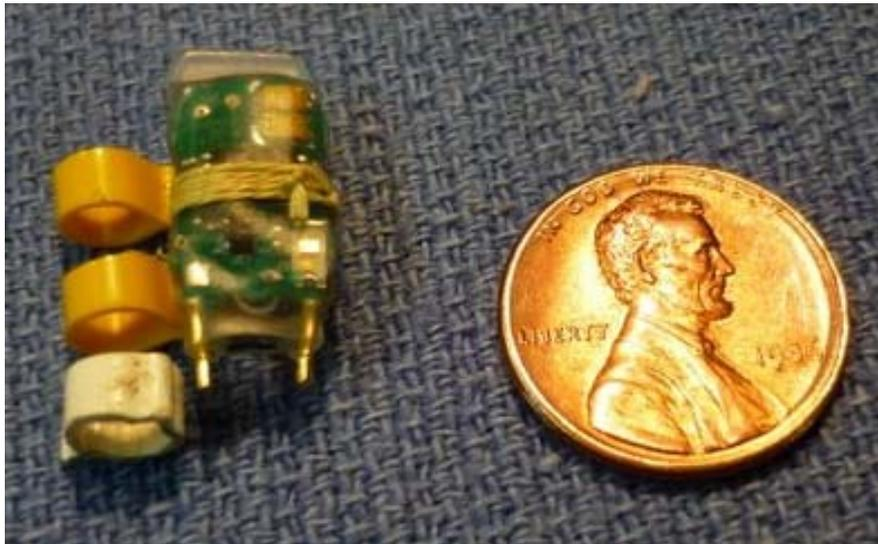
**Figure 9 – Example of a specially made plastic leg flag with two loops (for a wader). The white ring was included as a spacer above the leg joint and the pins were cut down further than shown here to reduce the risk of harm to the leg. The surfaces of the logger and plastic flag are first roughened with sandpaper to enable cyanoacrylate adhesive (superglue) to form a good bond after the thread is tied. Photo and details courtesy of Ron Porter.**
