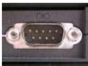
**Figure 20 - Serial RS232 9-pin D-type port**
