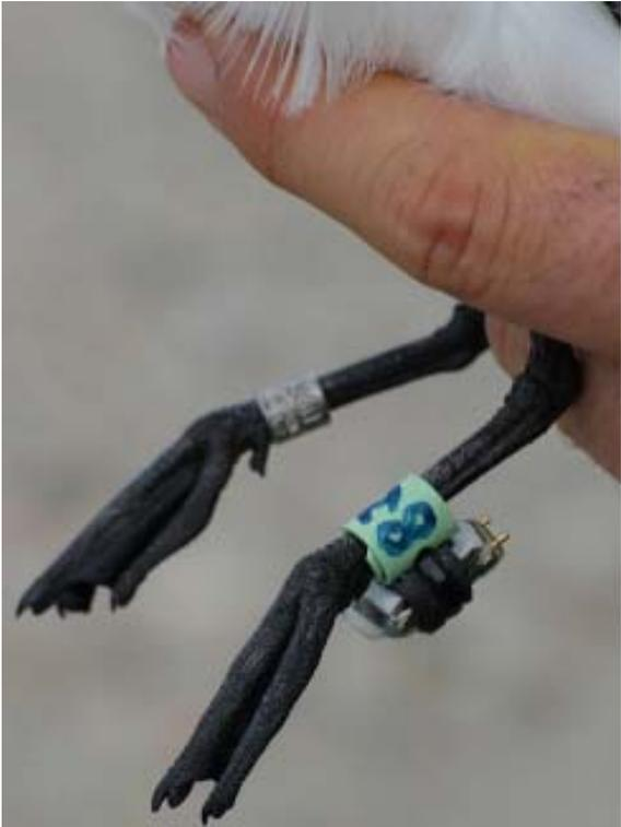
**Figure 11 – Example leg mounting of a Mk10 on Sabine's Gull. Photo courtesy of Carsten Egevang.**
