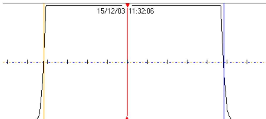
Figure 26 - Sunrises are marked with a yellow vertical line and sunsets with a blue vertical line. The red line shows your current cursor position and corresponds to the time shown above it. The data shown here is ideal with no visible interference near sunset or sunrise; the confidence figures assigned should be high.
